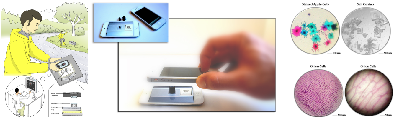
Figure 1: (Left) Illustration of our cellphone microscope in the field. The data captured by this versatile and low-cost platform can either be analyzed directly on the phone or remotely, for instance by a medical doctor in a hospital. (Center) Our prototype consists of a standard cellphone camera, a secondary lens on a mount that is directly placed on the microscopic sample, and background illumination, for instance provided by an LED or a secondary cellphone display. Optical magnification is achieved by mounting a small lenslet at its focal length to the sample. (Right) Microscopic images showing stained apple cells, sea salt crystals, and onion cells.
